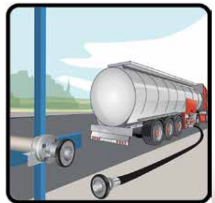
No spillage or damage after the coupling has break apart.
