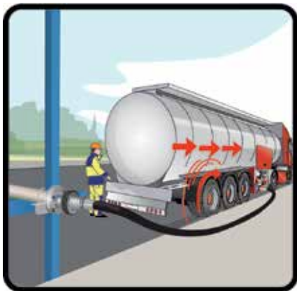
If the vehicle starts to roll away during loading / unloading serious incidents can happen if no Safety Break-Away coupling is installed.
